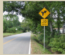
Curve Warning Signs with Advisory Speeds ($)
