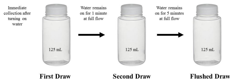
FIGURE 9. WATER SAMPLING PROCEDURE FOR METALS
